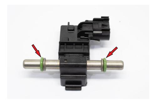
Insert one end of the flex sensor into the larger half of the bypass at a 90deg angle as shown below, gently twist while inserting to avoid pinching the o-ring.
