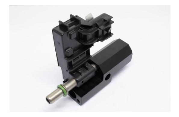
Lubricate the small o-ring on the smaller half of the bypass with a smear of engine oil.
