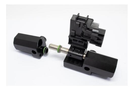
Insert the other end of the flex sensor into the smaller half of the flex sensor, gently twist while inserting to avoid pinching the oring. Once the o-ring is no longer visible line the smaller o-ring up with the hole in the larger half of the bypass, keep pushing the halves together until seated.
